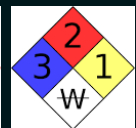
NFPA Code 704 chemical hazard label
