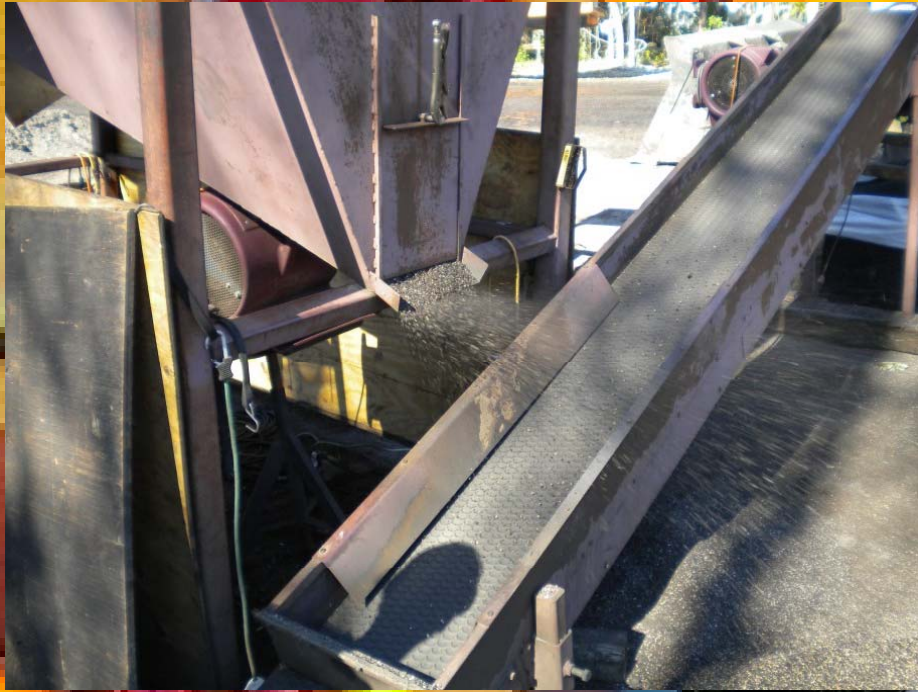
Separation of shot from similar mesh-size debris
